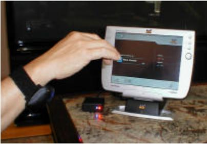
Figure 2. A/V Display w/ controller and USB base station
